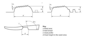
The diagram above explains the minimum requirements of the components of the sole
